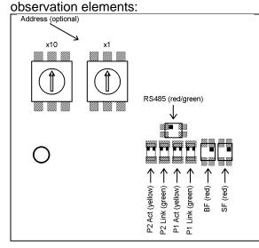
The LEDs are visible through two windows even when the bus adapter cover is closed.
