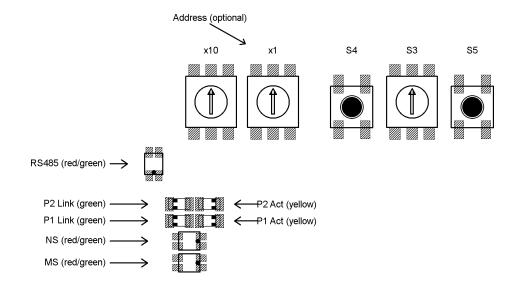
The LEDs are visible through two windows in the housing cover even when it is closed.
