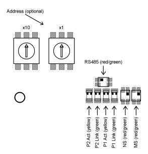
The LEDs are visible through two windows even when the bus adapter cover is closed.
